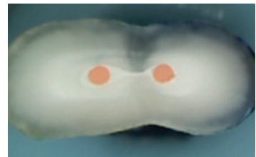
Optical microscope image of microleakage test (dye penetration test) ; No dye penetration
