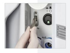
High capacity data logger The 8 gigabyte USB drive
